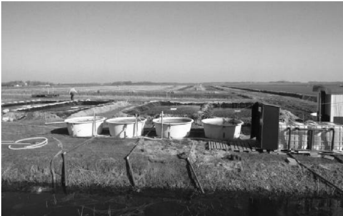
Figure 4. Test facilities on Texel. On the foreground the four 2 m 3 mesocosms, behind the four 25 m 3 ponds. In the background the Eversteekoog constructed wetland
